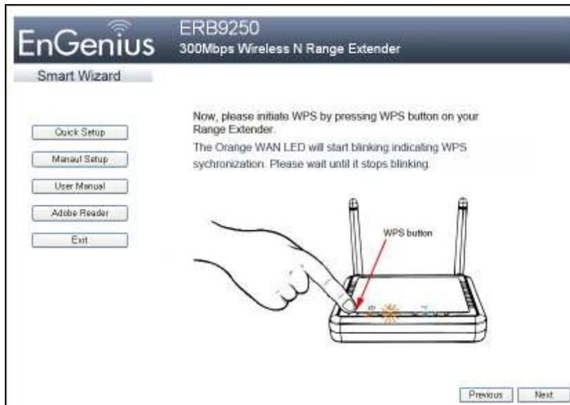
8. Press the WPS button on the front panel of your Range Extender once. The orange LAN LED (
