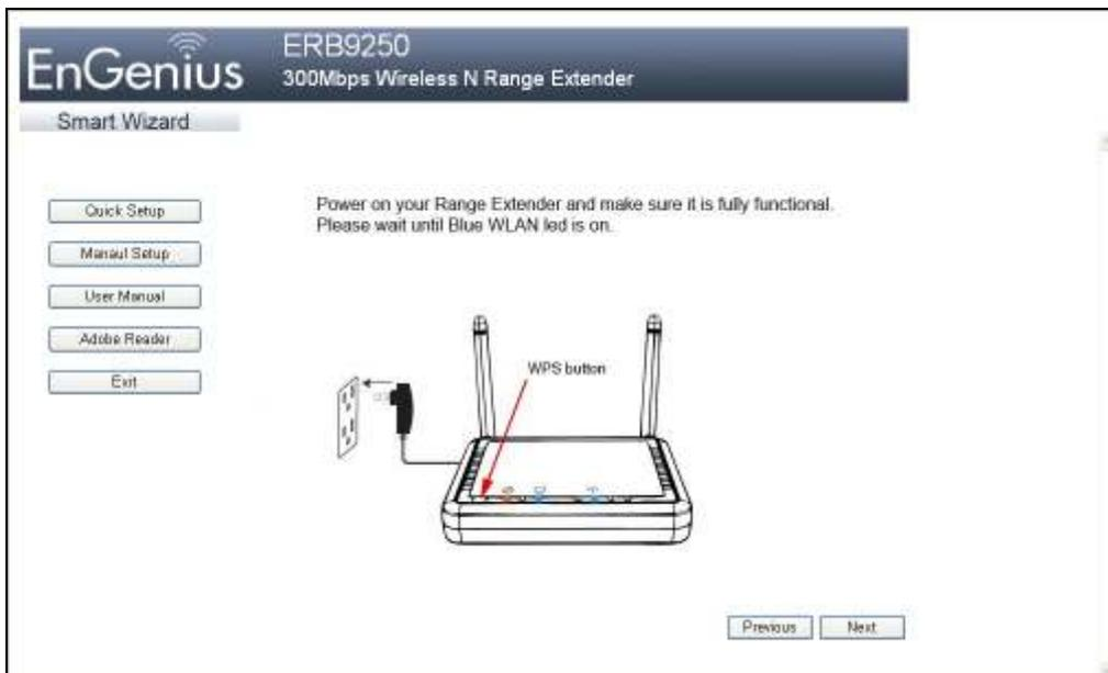
7. Attach the supplied power adapter to the rear panel of your Range Extender to power on the Range Extender and wait for the blue WLAN LED (
